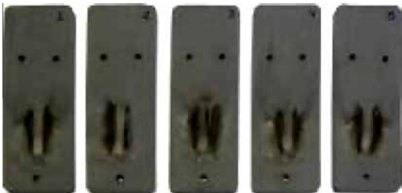
Fig. 10. Samples after electrical tracking and erosion tests in AC (steady method).
