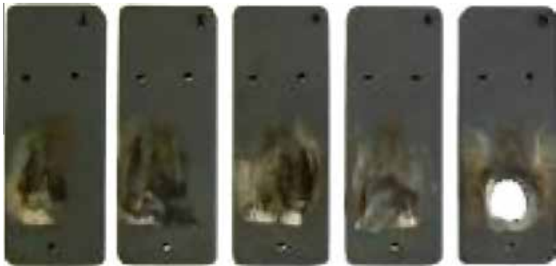
Fig. 7. Samples after electrical tracking and erosion tests in AC (step method).
